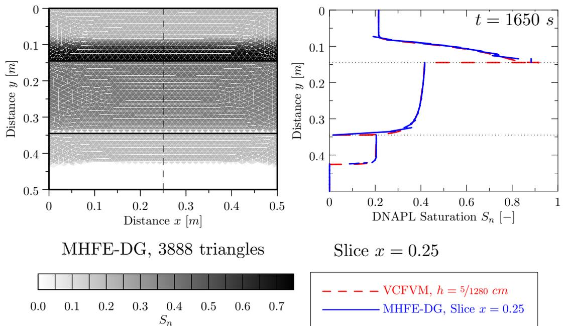
Figure 6: Numerical solutions of the barrier effect test problem using the MHFE-DG method in 2D. Slices of the numerical solution at  $x = 0.25$  are compared to the numerical solution obtained using the VCFVM in 1D on a very fine mesh. The time step  $\Delta t$  is chosen adaptively.
