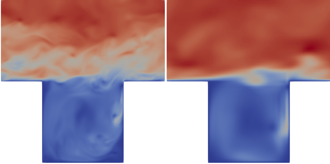
Figure 2.3: The effect of SVV in our simulations with parameters m = 0.75P (left) and m = 0.1P (right) on velocity magnitude at Re = 9000 .
